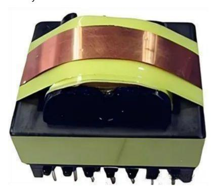
3. The primary winding is placed in the innermost layer of the transformer, and all the outer winding can screen this layer. This method mainly considers that the drain of MOS tube produces unstable voltage, which affects the primary coil.
